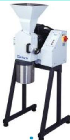
Figure 12. Knife grinder used for the sample prep (RETSCH, SM-2000)
