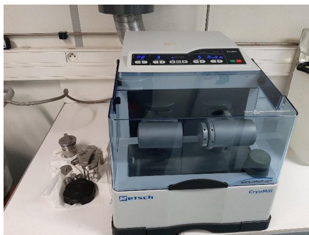
Figure 14. Cryogrinding apparatus (RETSCH Cryomill)
