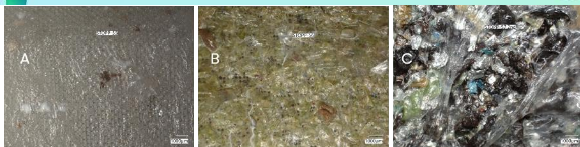
Figure 9: Close-ups of melt-filters (task 5.2 feedstock). A PP caps Germany, B separated Finland, C separated Germany
