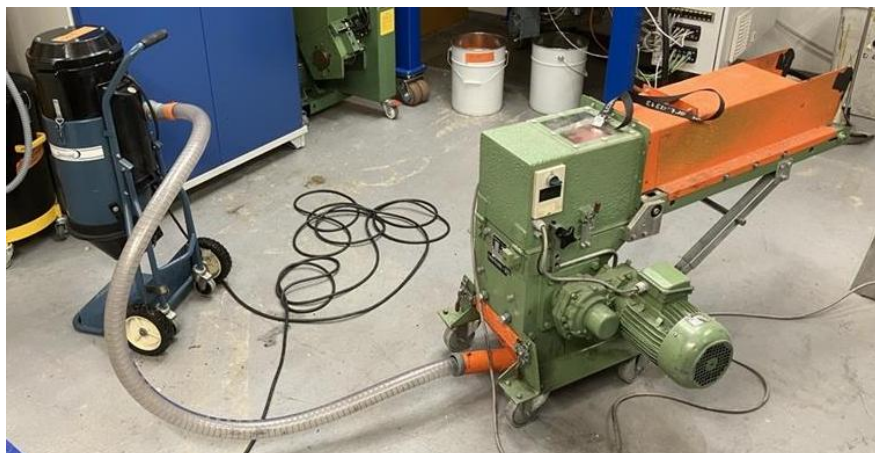
Figure 5: Pilot-scale grinding setup at VTT, used for size reduction.
